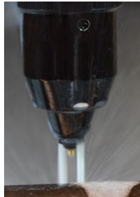
With high pressure internal coolant
