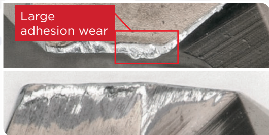
After drilling 900 holes
